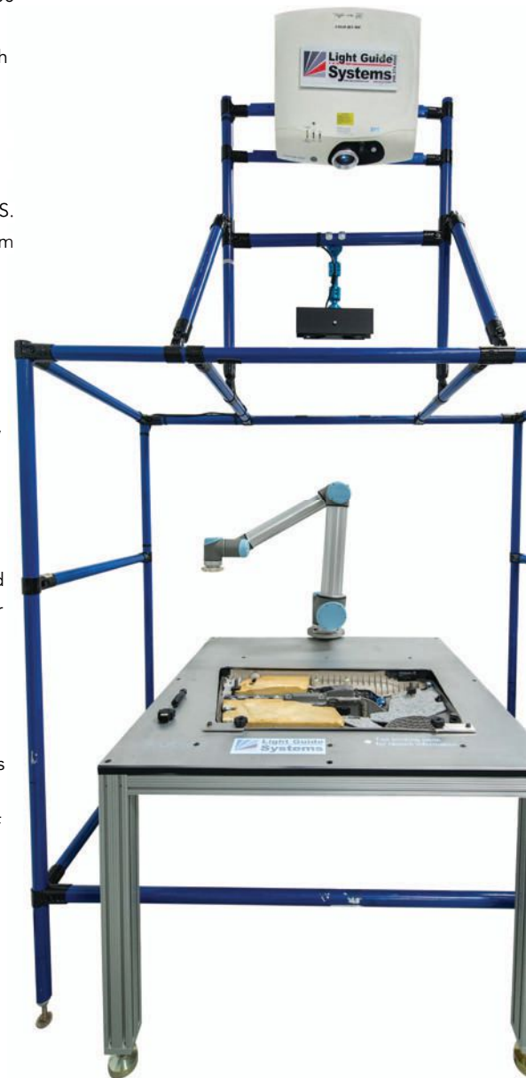
OPS Solutions' Light Guide Systems simplifies complex manual tasks by having equipment operators follow illuminated signals.
