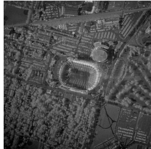
Figure 3: SAR X-Band image of the University of Michigan Stadium collected by Maxar Intelligence's Data Collection System (DCS) testbed at 1ft resolution. Copyright 2024, Maxar Mission Solutions, Inc
